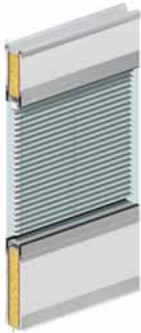
Part double glazed vertical section with integral venetian blinds
